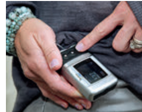
An artificial pancreas algorithm refines the dosage administered through an insulin pump, above, with the tightest possible glucose control and the least hypoglycemia and hyperglycemia.
